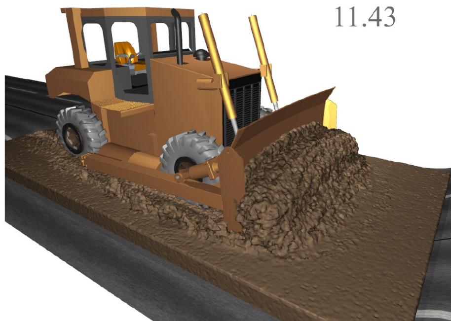
Figure 1.1. Combined multibody dynamics/DEM model of a bulldozer performing an earth leveling operation on mud
